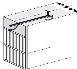
When installing, centre the assembly in relation to the garage door.
