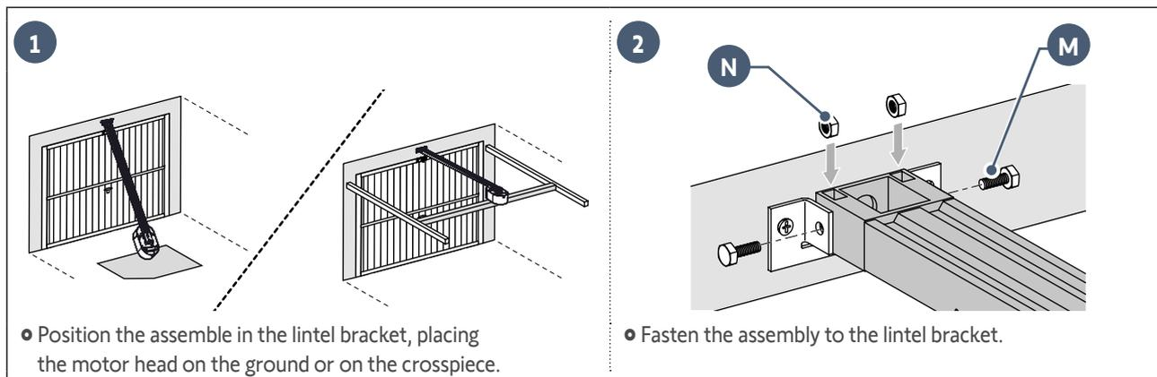
> Mounting the linking arm on the door and the carriage
