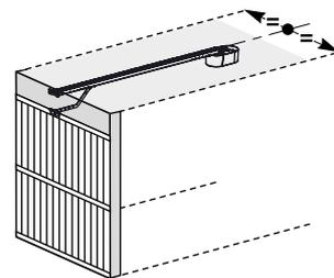
When installing, centre the assembly in relation to the garage door.
