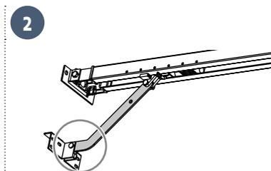
The part of the linking arm fastened to the door bracket must be as horizontal as possible.
