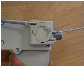
Fig 1. Removal of QR cover.
