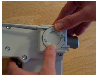
Fig. 3. Replacement of QR cover.
