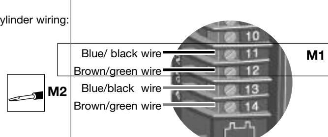
**⚠ The cylinder M1 is always connected between terminals 11 and 12.
