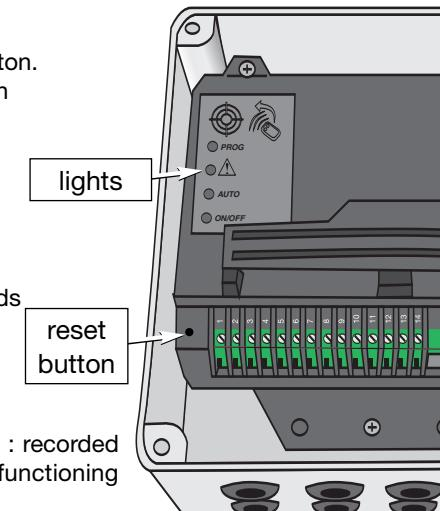
All the recorded parameters are deleted : recorded remote control, gate displacement, functioning mode...
