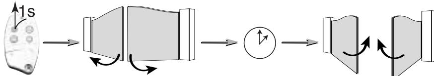
It is possible to maintain the gate in the open position by giving a stop order (push again on the remote control button) :
