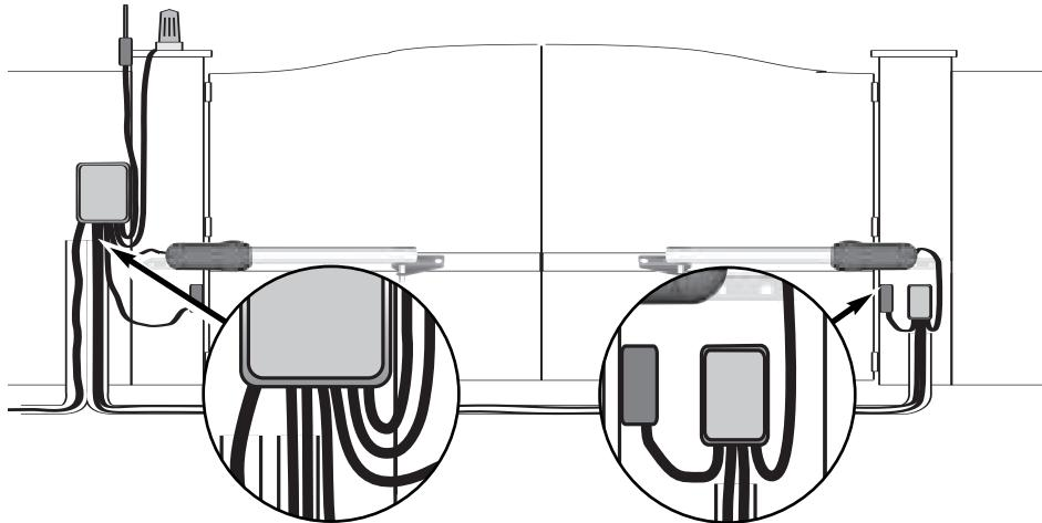
Attach the switch box on the pillar.
