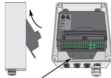
The box will be mounted with the stuffing box towards the bottom.
