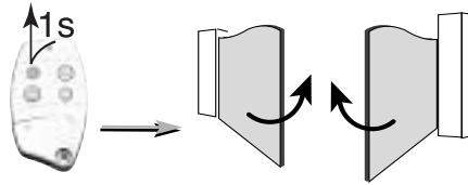
At the end of these 4 steps, the PROG light turns off, indicating the end of the gate displacement memorization procedure.
