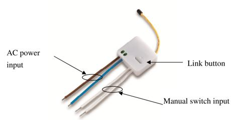
HAC01 can be installed into the in-wall power box, the power cord have to be connected to the main AC power, the manual switch input cable is wired to normal NO (open) / NC (close) button or switch. When the wiring connection is completed, please follow the previous instruction to operate the Inclusion and Association process to finish HAC01's connection and network setting with controlled device (ex. HAN01).
