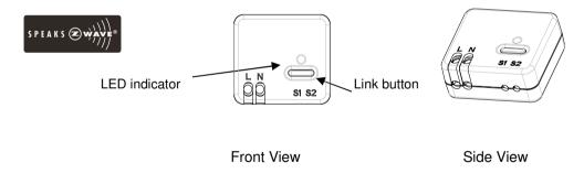
When first power is applied, the LED flashes on and off alternately and repeatedly at 2-second intervals. It implies that it has not been assigned a node ID and cannot work with Z-Wave enabled devices. Please get familiar with the terms below before starting the operations.
